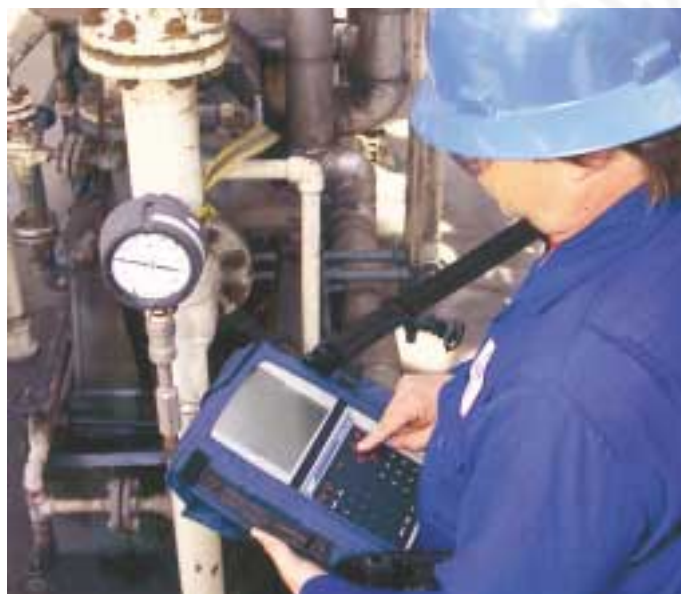
Microlog – portable data collector and analyser
